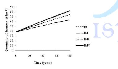
Figure 2a: K2 = 0.005T0:  $Y = -203.27e^{-0.005x} + 241.15$ ; R-sq = 0.977TM:  $Y = -144.16e^{-0.005x} + 182.04$ ; R-sq = 0.984TMA:  $Y = -242.21e^{-0.005x} + 280.10$ ; R-sq = 0.973TMM:  $Y = -247.01e^{-0.005x} + 284.89$ ; R-sq = 0.972
