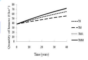
Figure 2b : K2 = 0.01T0:  $Y = -82.69e^{-0.01x} + 120.57$ ; R-sq = 0.973TM:  $Y = -53.14e^{-0.01x} + 91.02$ ; R-sq = 0.981TMA:  $Y = -102.17e^{-0.01x} + 140.05$ ; R-sq = 0.969TMM:  $Y = -104.56e^{-0.01x} + 142.45$ ; R-sq = 0.968
