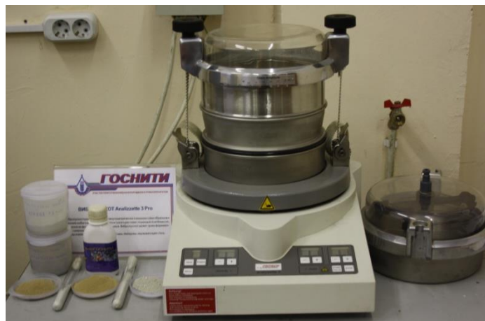
Figure 1: Fractionation of powders in a vibrating screen «Analysette 3 Pro»; the powder left is the original; in the center – processed, it became lighter; right powder companies «IKSAR»; in vials tribo-active «Sarnowski» and «RVD»; in jars powders CFG from Georgia
