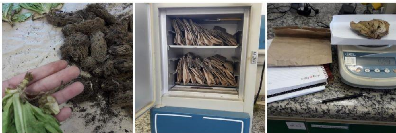
Figure 06: Illustration of the steps to obtain the dry weight of the aerial part of greenery. Source: Nathalia Hiratsuka.
