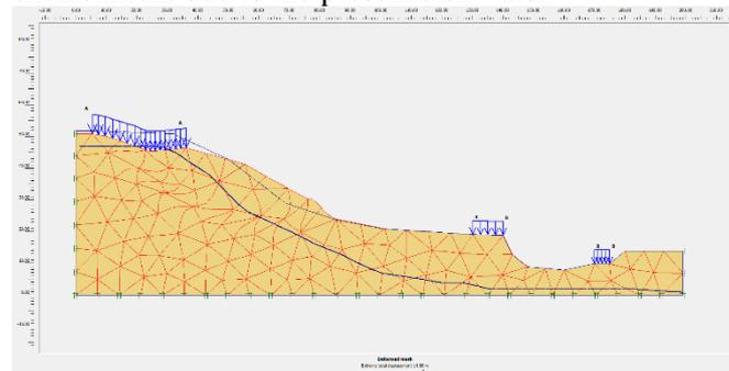
**Figure 11. Deformation of the environment due to the presence of water**
