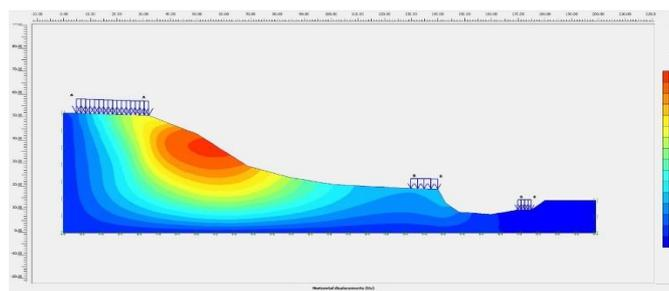
**Figure 7. Vertical displacement in dry state without structural element**
