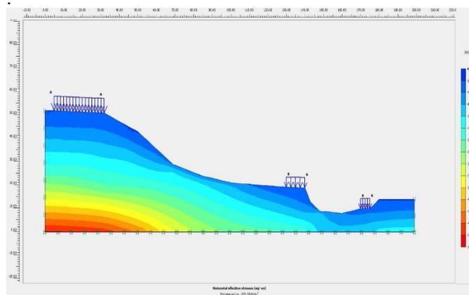
**Figure 5. Horizontal effective stress in dry state without structural element**
