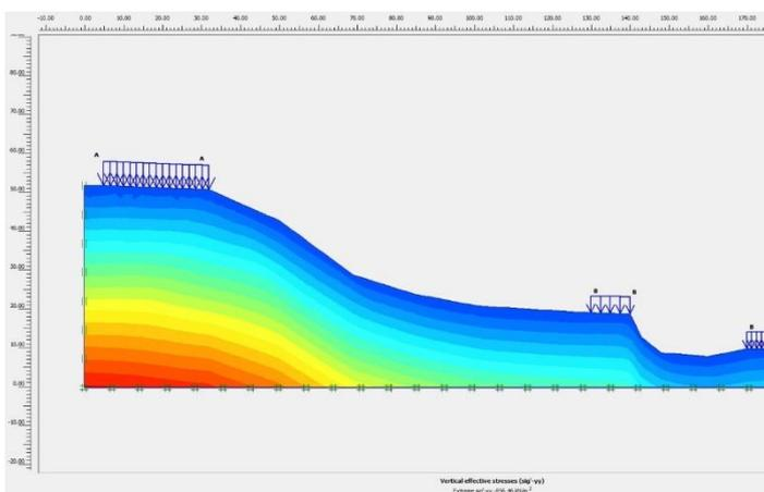
**Figure 9. Vertical stress in dry state without structural element**
