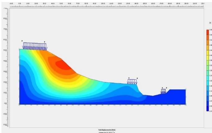
**Figure 8. Total displacement in dry state without structural element**
