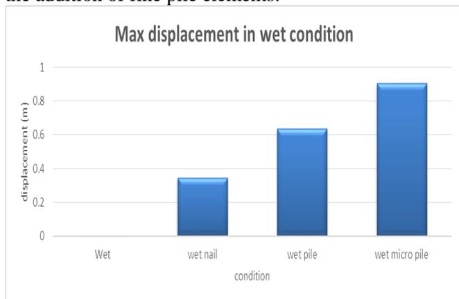
**Figure 14. Comparative total displacement in seepage mode**
