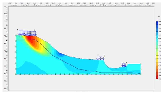
**Figure 12. Vertical displacement in case of water seepage**
