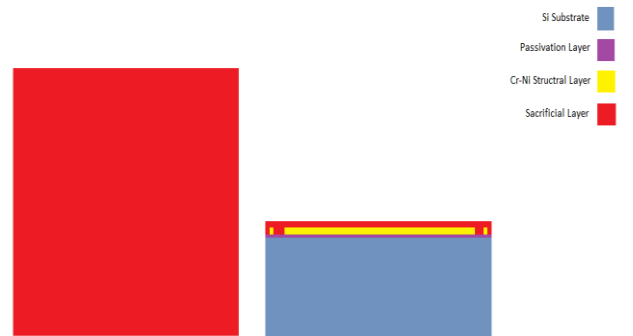
Figure 27. Sacrificial layer of the first stage
