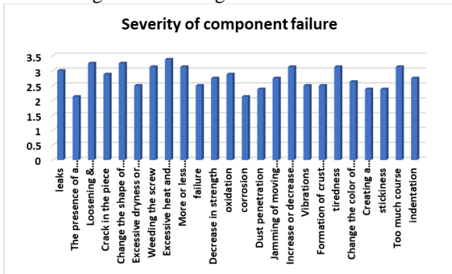
Figure 6. Damage severity of machine parts based on FMEA
